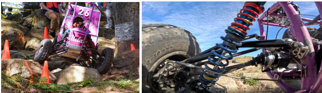
Figure 25. (a) Top shows the UCA (painted black) fulfilling all geometric design requirements. (b) Bottom shows the Baja SAE vehicle completing the Oregon competition rock crawl, the most suspension-taxing competition event.
