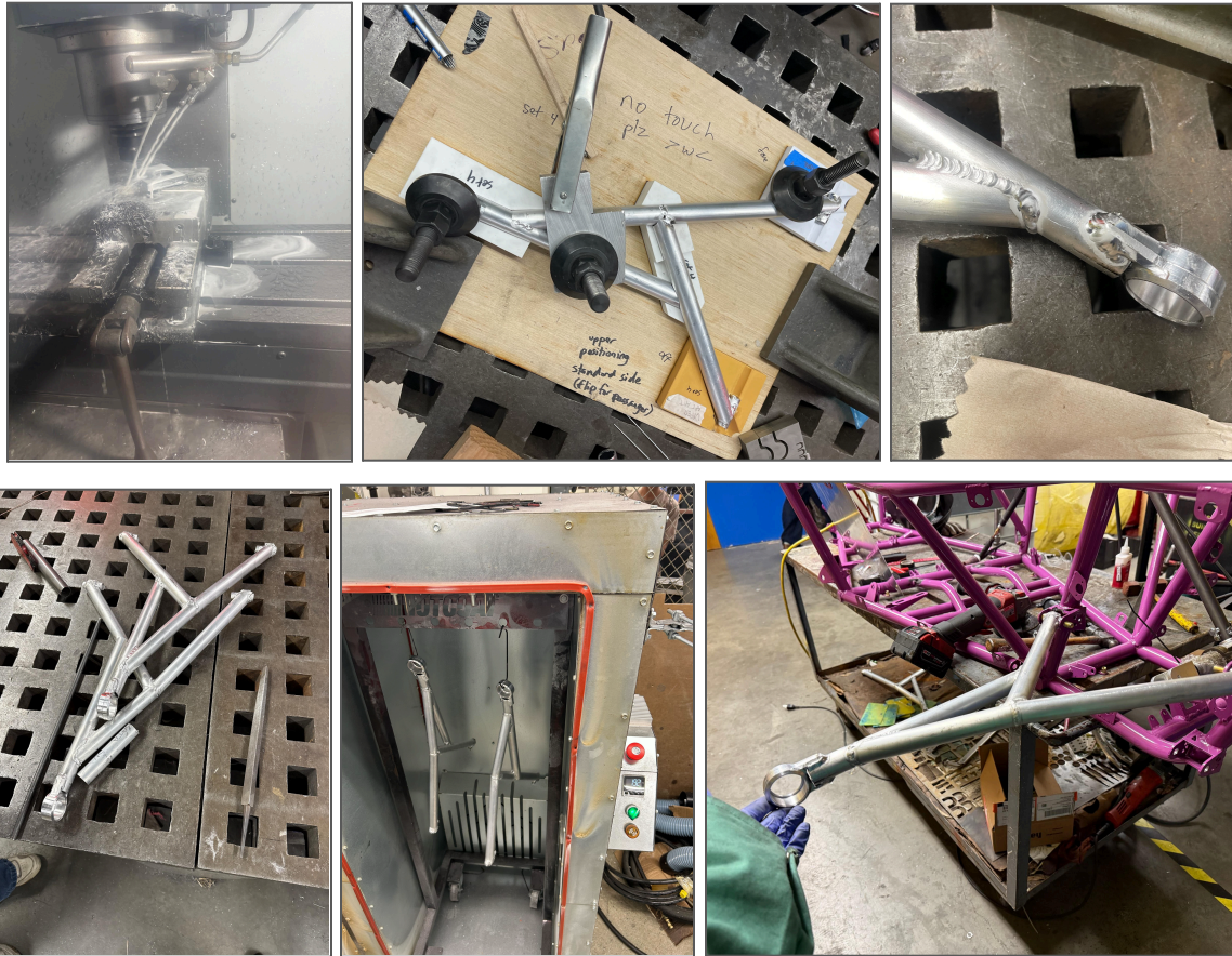
Figure 23. Manufacturing process. (a) top left shows the wafer CNC process. (b) top middle shows the jigging system. (c) top right shows part of the welding process. (d) bottom left shows the fully welded arms. (e) bottom middle shows the heat treatment step. (f) shows the finished product on the Baja SAE vehicle.
